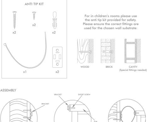
1. Mark the location of the hole on the wall using bracket approx 1" below the top of furniture. Predrill the holes at parket location & insert wall plug. Align bracket onto wall plug & secure using long screws.
